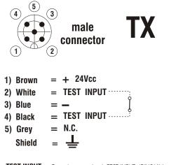
$\begin{array}{l} \textbf{TEST INPUT} = \text{Opening contact TEST INPUT (PIN2/4) is simulated} \\ \text{the interruption of the curtain and testing the correct opening} \\ \text{of the outputs SW1 - SW2 of the receiving unit} \end{array}$
